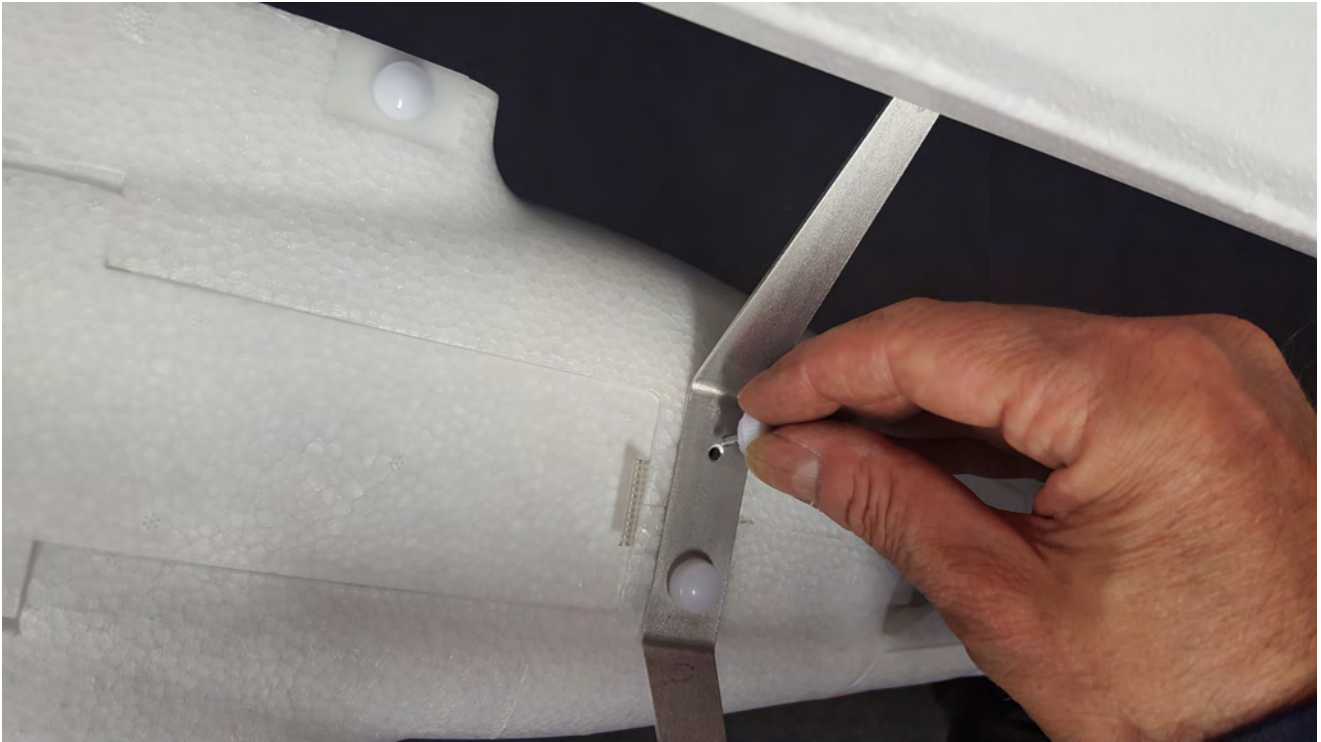
Step 4: Attach the floats with the 4 supplied thumb screws
